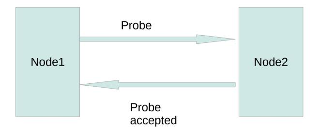
Node 1 and Node 2 are peers in a trusted storage pool
