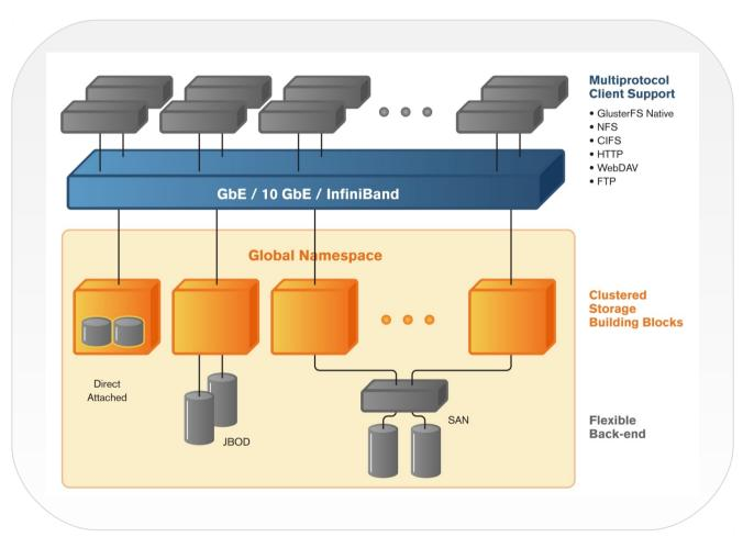
**Global namespace Scale-out** storage building blocks **\$**Supports thousands of clients Access using **GlusterFS** native, NFS, SMB and HTTP protocols **C**Linear performance scaling
